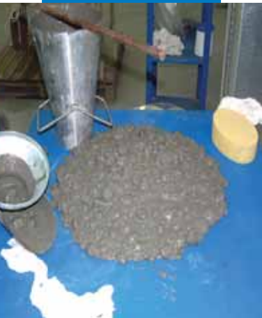
Appearance of concrete after initial slump test
