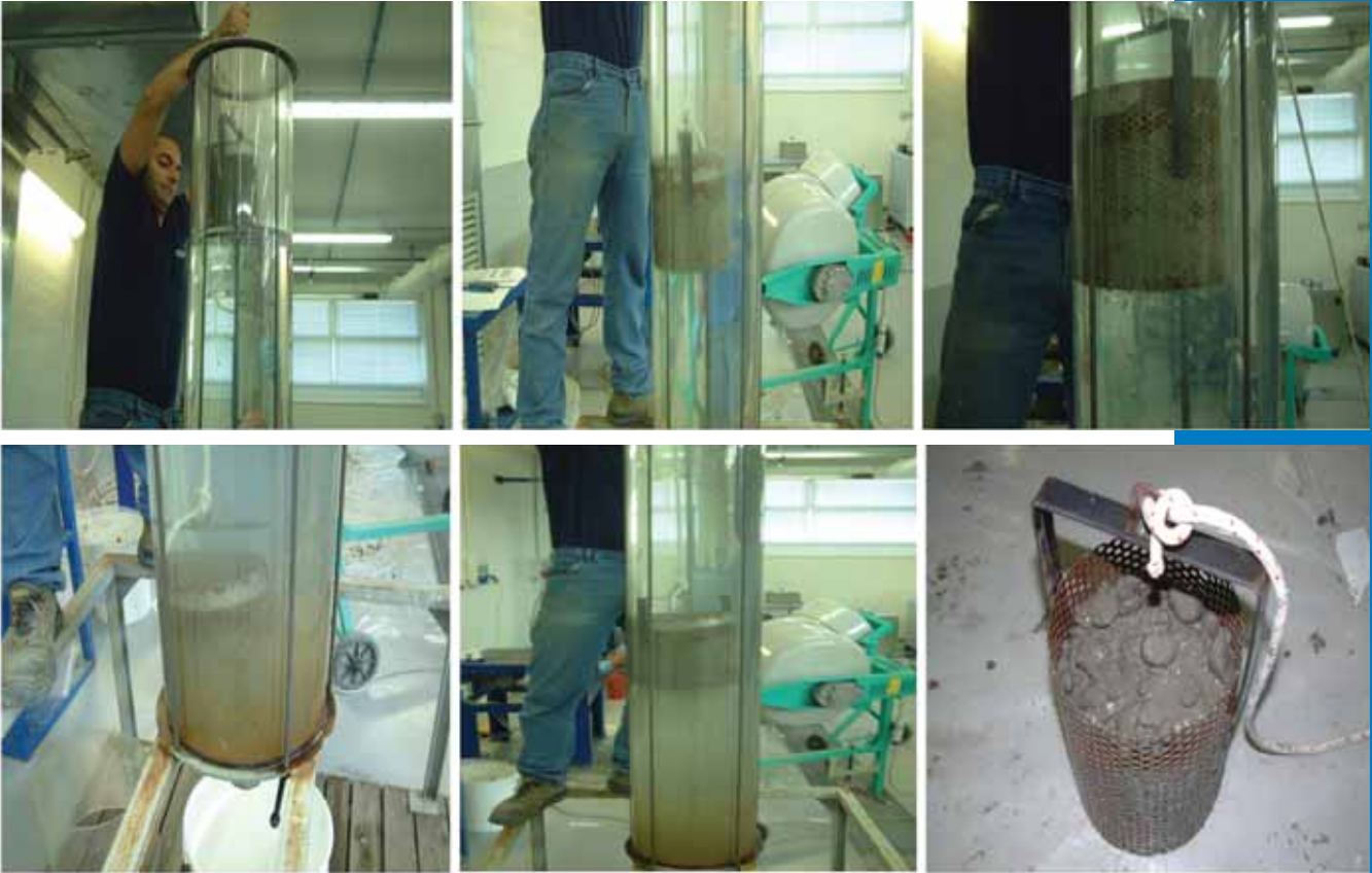
Assessment of leaching and appearance of concrete after testing
